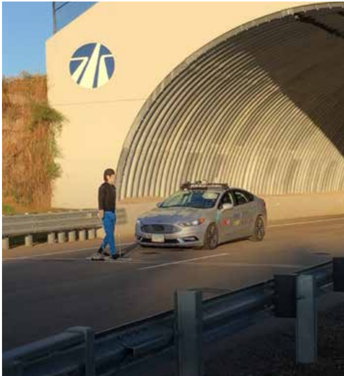
Tunnel Sunrise Dazzle gap test setup
