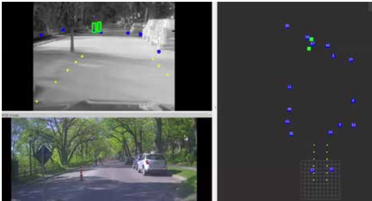
Fused thermal and radar (top left), visible (bottom left), green represents thermal in the radar field of data (right)
